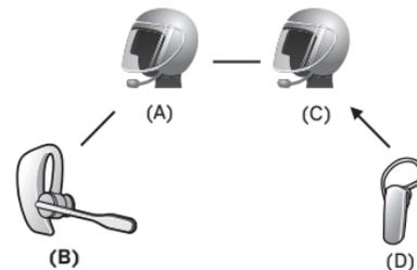
4. Now two SC1 headsets (A & C) and two non-Sena Bluetooth headsets (B & D) are connected with the four-way Universal Intercom.
